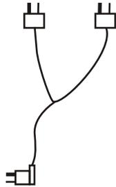
One of the pins is thinner than the other. Accordingly, on the hearing aid too, one hole is smaller than the other. The thicker pin goes into the larger hole, and the thinner pin into the smaller hole. Do not unplug the cord unnecessarily, as the cord and the pins will begin to show signs of wear and tear.
