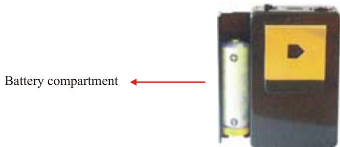
While inserting the battery into the battery compartment, check that the positive terminal of the battery (marked with +) is in contact with the positive
