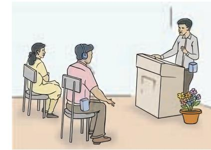
Personal Listening Devices are usually based on FM technology. These are typically used in schools, meetings, discussions, etc. The speaker wears a microphone that is either clipped on to their collar or as a headset. This is connected to a transmitter, which sends out FM signals to the receiver. The receiver wears ear buds, or earphones on a headset. Personal Listening Devices can also be carried around in the
