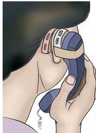
**b. Add-on amplifier:** This type of amplifier can be attached to the receiver end of the existing telephone. It can be removed from the telephone. The biggest advantage of this amplifier is that it can be used with different phones. The user may even carry the add-on amplifier around and use it when he/she uses public/other phones. These amplifiers are also cheaper and easy-to-use. However, they may not work with all phones. Also, batteries need to be changed regularly.
